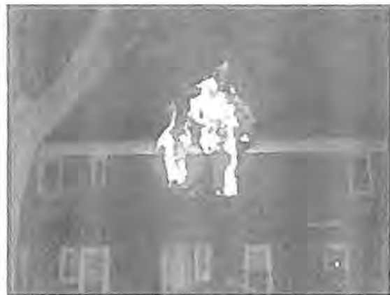
Figure 4-12: Structure fire after flashover has occurred.
