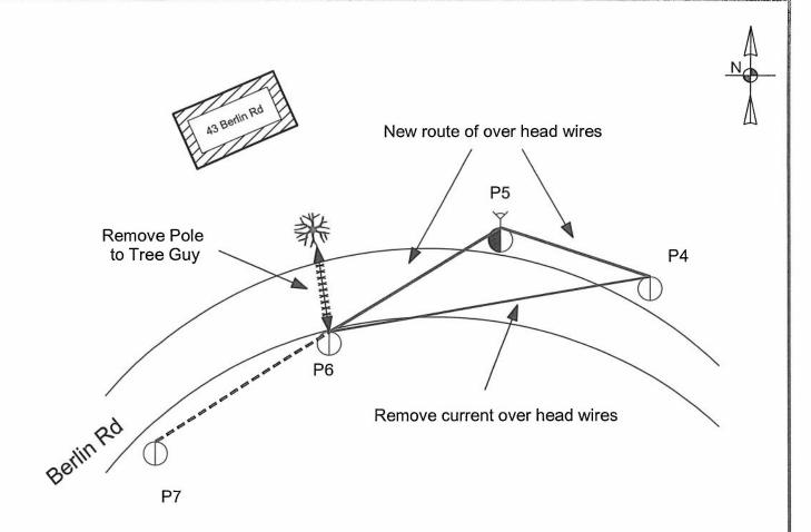
Install new pole #5 and anchor This will allow the removal of the pole to tree guy at 43 Berlin Rd
