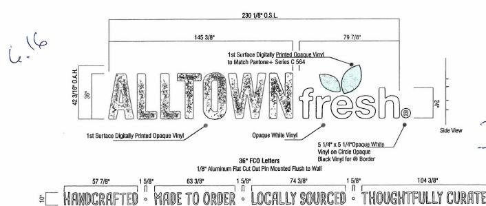
10" FCO Letters 1/8" Aluminum Flat Cut Out Pin Mounted Flush to Wall
