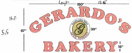
(1) set of 15"x 5.5" Channel lit raised letters. White aluminum cabinets (040 gauge) with diabond backing. Red translucent film on white signgrade acrylic letters, black plastic trimcap. LED lighting, all UL listed wiring devices.
