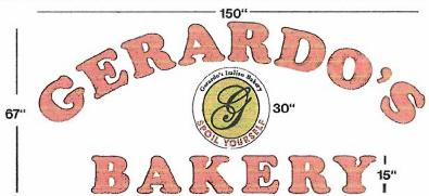
(1) set of 15"x 5.5" Channel lit raised letters. White aluminum cabinets (040 gauge) with diabond backing. Red translucent film on white signgrade acrylic letters, black plastic trimcap. LED lighting, all UL listed wiring devices.
