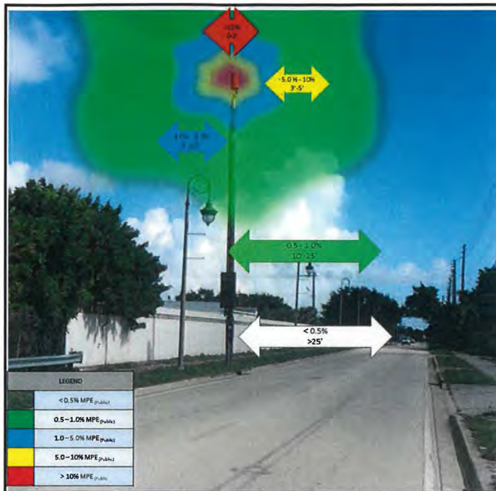
Figure 1: Results of RF field calculations for a typical AT&T antenna installation on a utility pole at 30' (AGL) showing profile view
