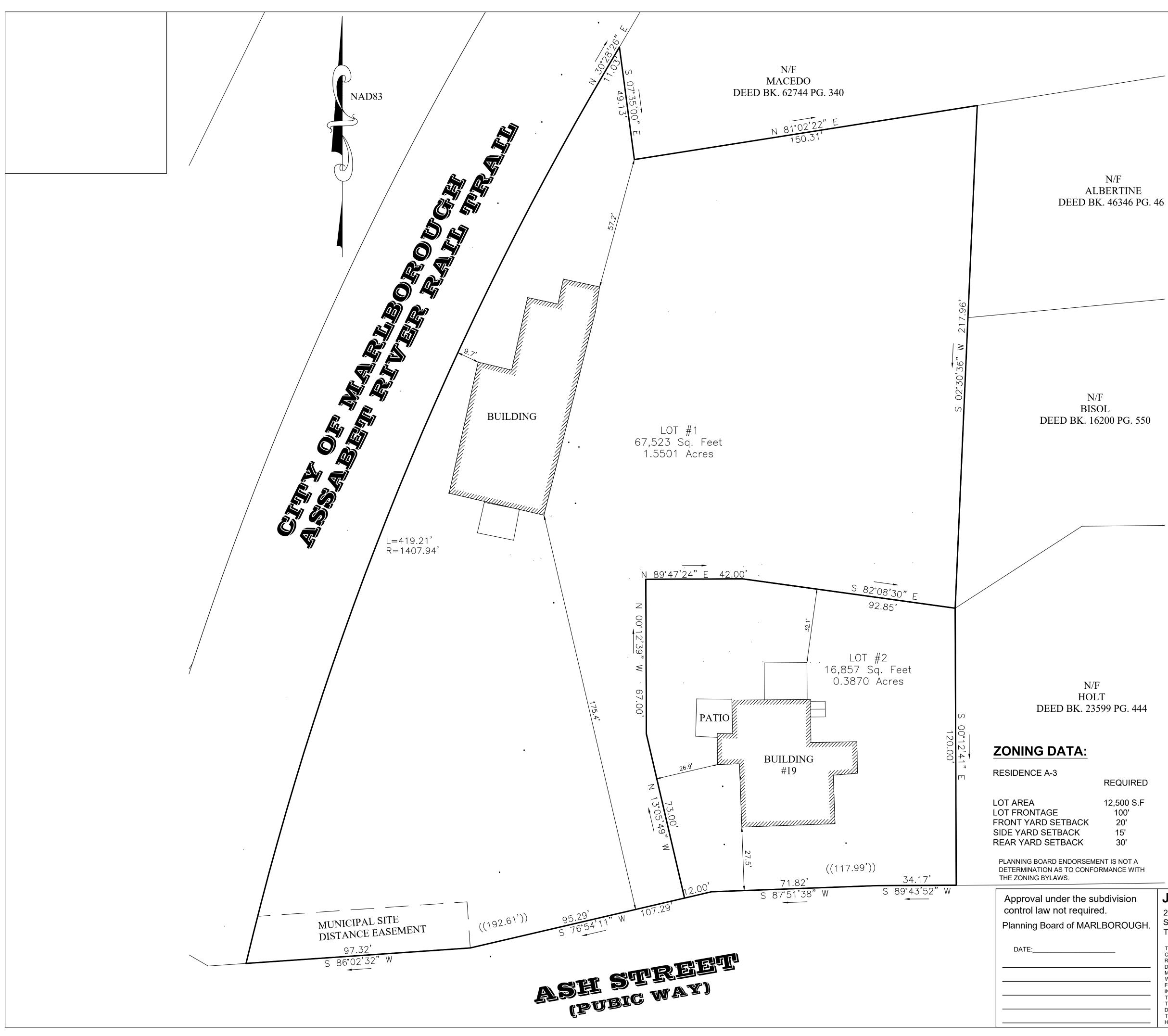
The purpose is to subdivide the existing 1.94 acres property, with a total of 310.60 feet of frontage on Ash Street into two lots; Lot #1 containing 67,523 sq. ft.\* of area with a total of 192.61 feet of frontage on Ash Street and Lot #2 containing 16,857 sq. ft.\* of area with a total of 117.99 feet of frontage on Ash Street.
