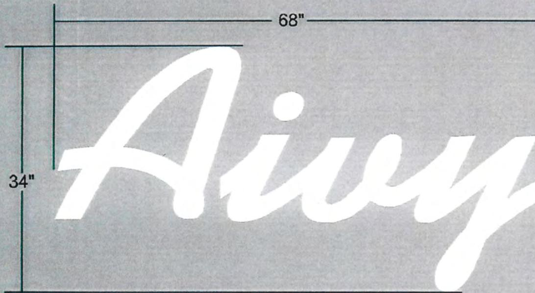
A)34"H x 68"W Channel Letters "Aivy": 5" matte white aluminum body/can with 3/16" thick white acrylic faces with 1" white trim. Internally illuminated with white LED. After removal of existing "Dalla" letters, individual letters will be mounted onto existing raceway.
